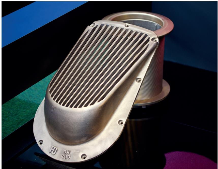
**1120F full grated water intake** is normally installed for toilets systems, as it lets water in with lower pressure. This is common also for round scoop 1210 and all the full grated scoops.
